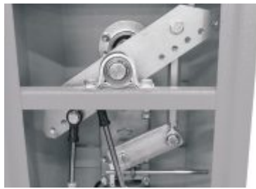
Double balance springs for smooth movement
